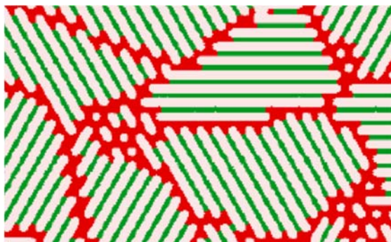
Schematic representation of the expected structure. White is crystal, and red and green are respectively the two amorphous phases with different compositions in A and B
